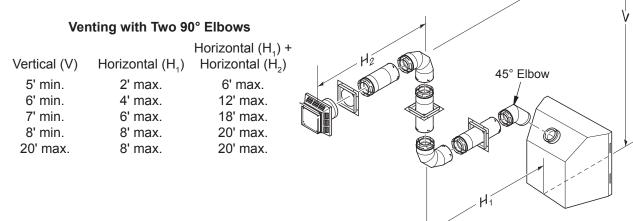
Figure 17 - Horizontal Termination Configuration for Venting Using Two 90° Elbows
